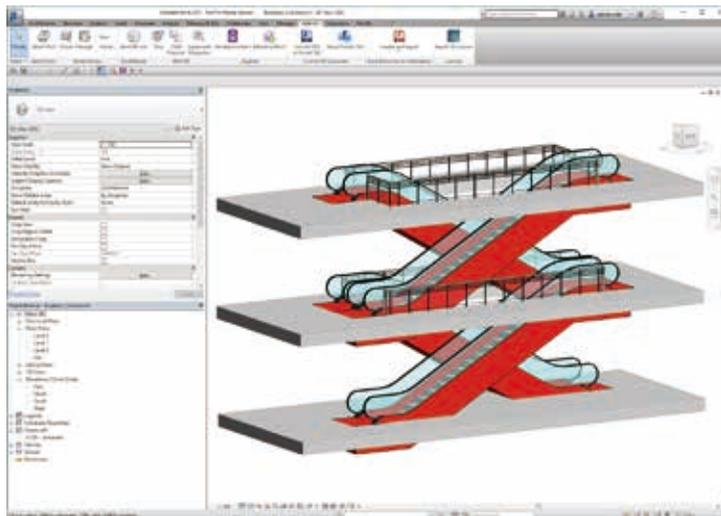
Schindler provides up-to-date planning tools for architects, planners, and consultants. 2D drawings and 3D models are provided by the DigiPara Elevatorarchitect plug-in for Autodesk Revit available at the Autodesk App Store.
